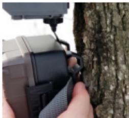
6. Mount your camera to the tree (the cable with SD adapter should now be placed between the tree and the camera.)
