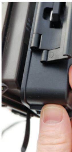
5. Run the cable behind the camera and upwards so that the end of the cable sticks out of the top of the camera, so that you can connect it to the CELL-LINK.
