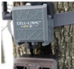
8. Plug the extremity of the cable with SD adapter to the CELL-LINK and screw it on tightly.
