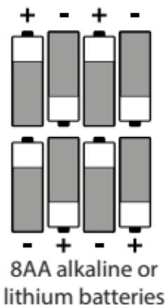
You can use any combination of the above power sources with your FORCE-48. If multiple power sources are connected, the camera will use them in the following order: 12V, and then the AA.
