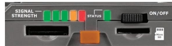
1. Make sure that your device is powered by new batteries and that a microSD card has been inserted.
