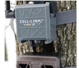
8. Plug the extremity of the cable with SD adapter to the CELL-LINK and screw it on tightly.
